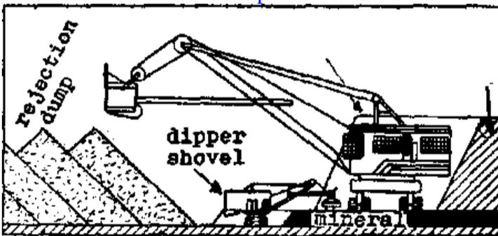
Fig. 5.10. -Quarry working with stripper and dipper shovels.
