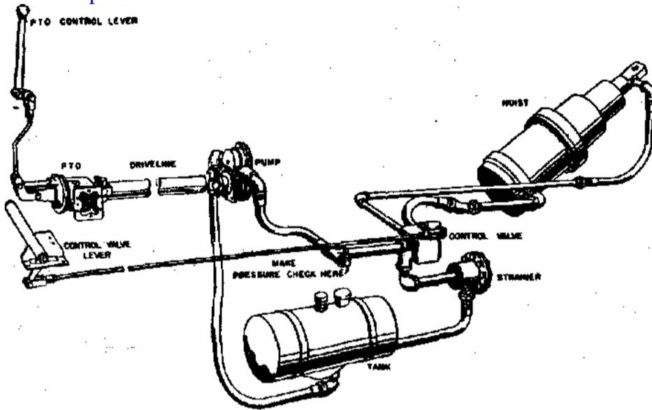
Fig.5.11 The tipping gear for dumpers
