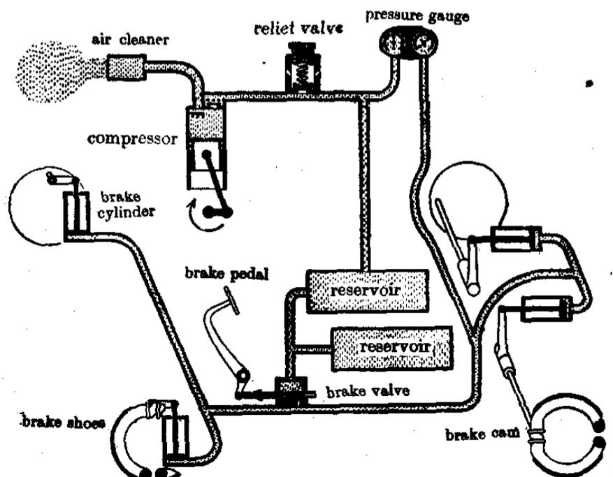
Fig. 5.12. Schematic arrangement of compressed air brake
