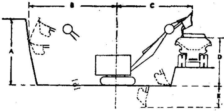
Fig. 5.7 A. Working ranges of a dipper shovel (maximum). Figures in brackets show the working ranges in m of Tata dipper shovel, model 1055 B, at a boom angle of 50°. Boom length is 8.53 m.
