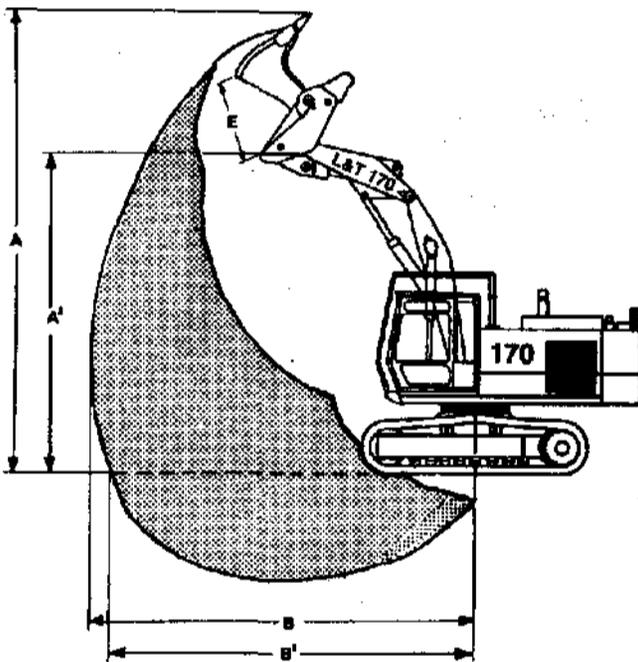
Fig. 5.8. Working ranges of L & T 170 CK-II bottom dumping shovel
