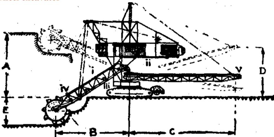
Fig. 5.2\$. General arrangement of a bucket wheel excavator
