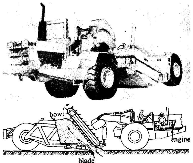
contents are unloaded in a layer 150 mm to 250 mm thick, over a distance of 30 to 70 m. The bowl is always bottom discharging. Scrapers are unsuitable in soils with stumps, large boulders and hard rocks. When the ground is hard, it is necessary to rip the surface with the help of a ripper before loading by a scraper. Sandy soil is best for a scraper which has to be stopped during rains, if engaged in alluvium. (Fig. 5.3).
