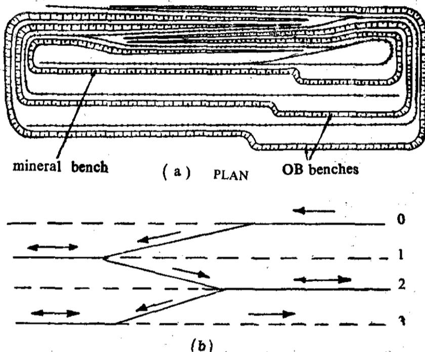
Fig. 5.20. Switch back layout (Vertical section exaggerated).
