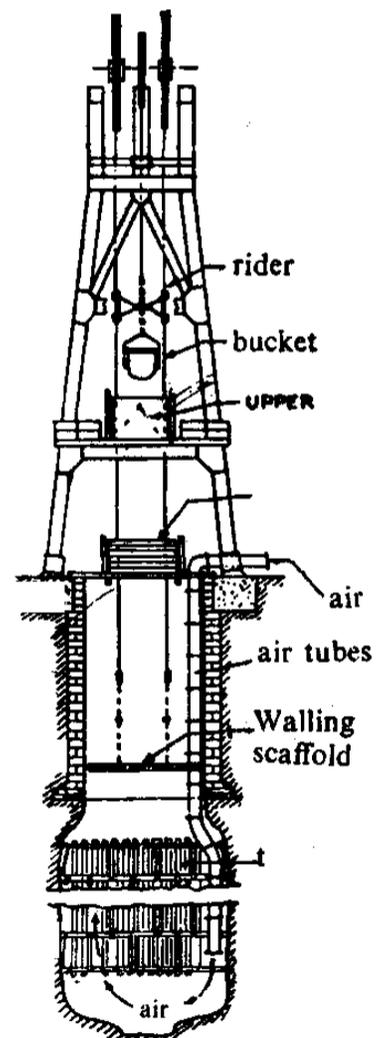
**General Arrangement of Sinking Shaft.**
