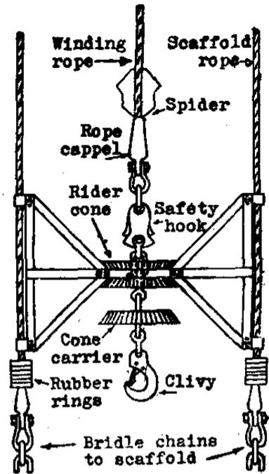
Fig. 4.6. Rider as used during sinking
