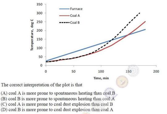
The results of the crossing point temperature experiments for coal A and B are shown in the figure.
