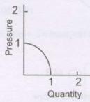
The combined characteristic of two such identical fans installed in parallel is
