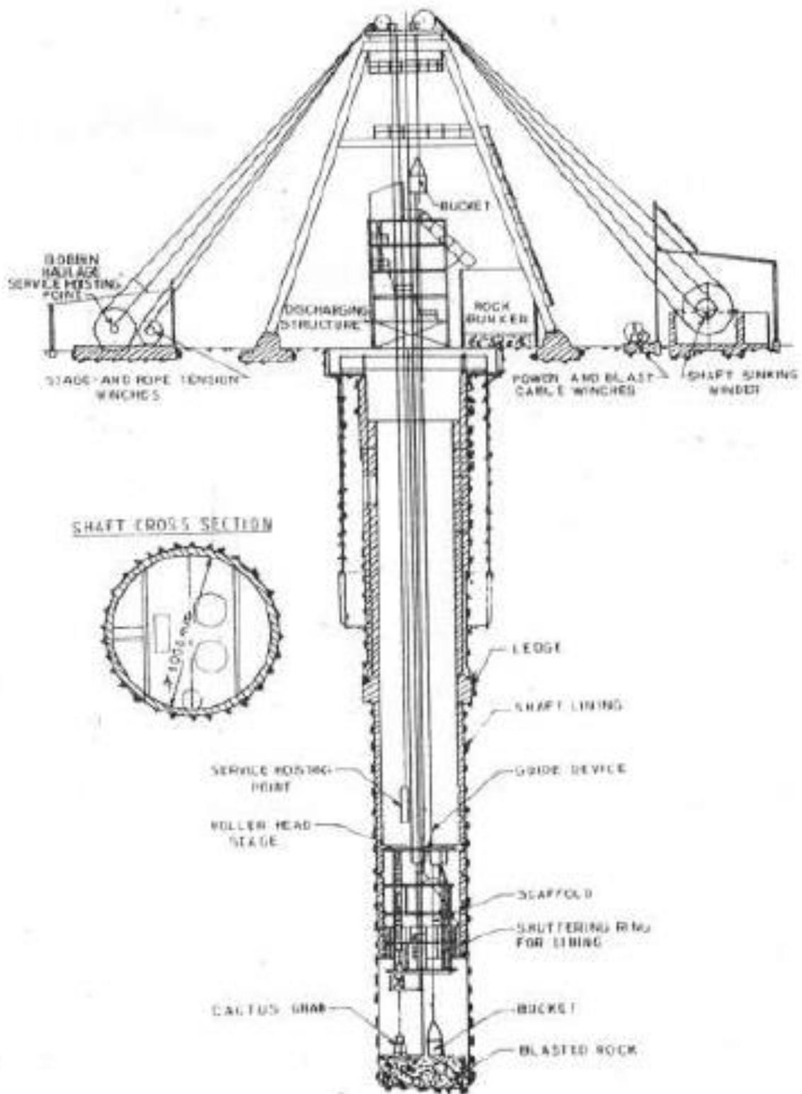
(GENERAL ARRANGEMENT OF SINKING SHAFT)
