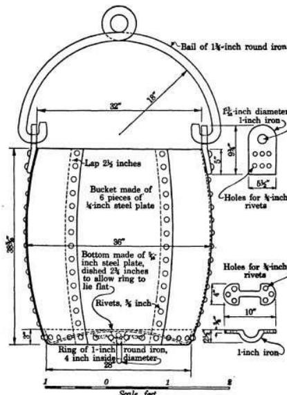
FIGURE —Nineteen-cubic-foot sinking bucket
