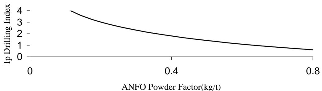
**Figure-5: - Correlation between I<sub>p</sub> drilling index and Powder factor**
