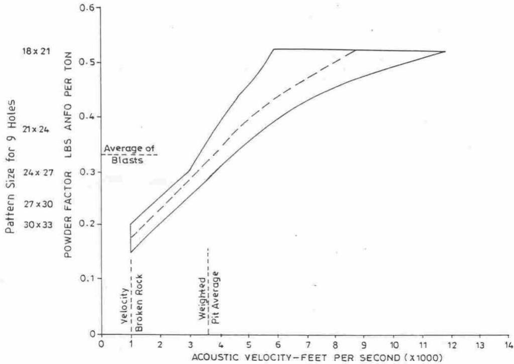
Figure - 2: Heinen & Dimock's correlation between fragmentation Vs powder factor, pattern size, and velocity
