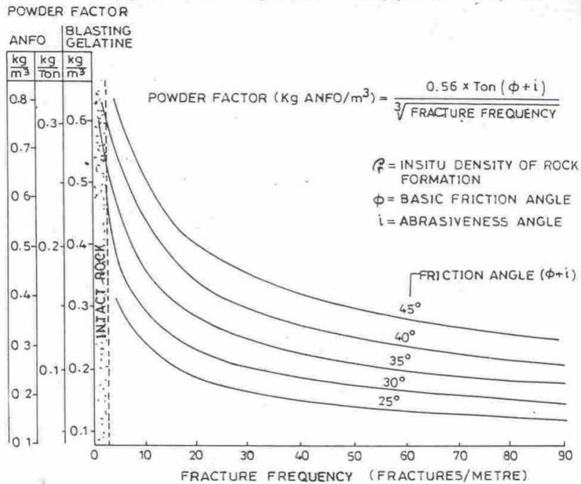
Figure - 3: Empirical relationship between powder factor, fracture frequency and joint shear strength, as proposed by Ashby
