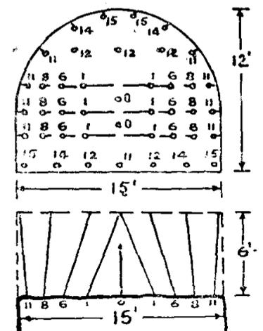
Fig. 2. Milli-second Delay Blasting with Wedge Cut.
